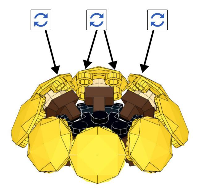
Rotate every other round plate, so that one stud points to the top. Alternate between, one pointing to the top, and two pointing to the top. Like this, the studs can interlock
