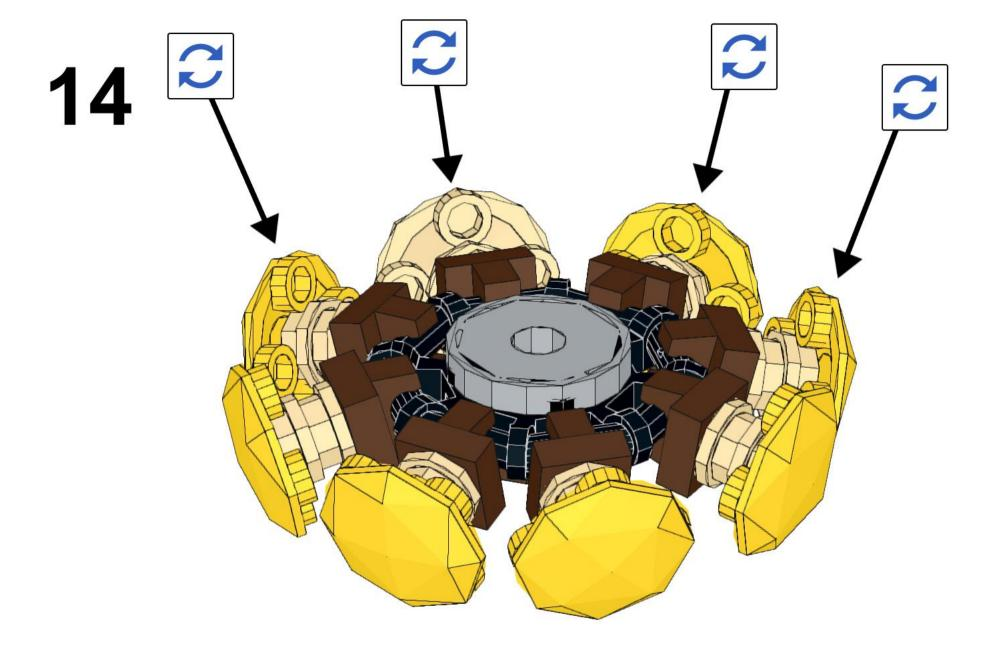
Rotate all round planes, so that always one stud points upwards.
